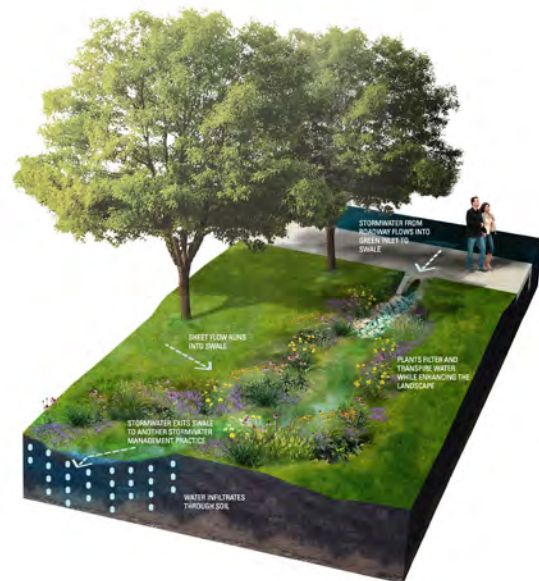
Diagrams of green stormwater infrastructure BMPs including stormwater planters and swales (Source: PWD / WRT)
